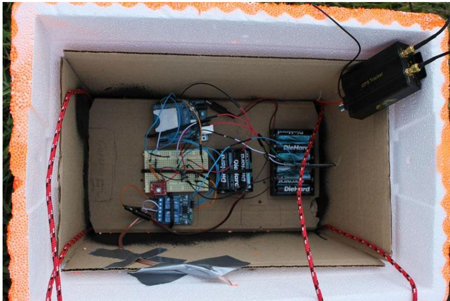
**Exhibit 1. Microcontroller and sensor components inside of the weather balloon payload box.**
